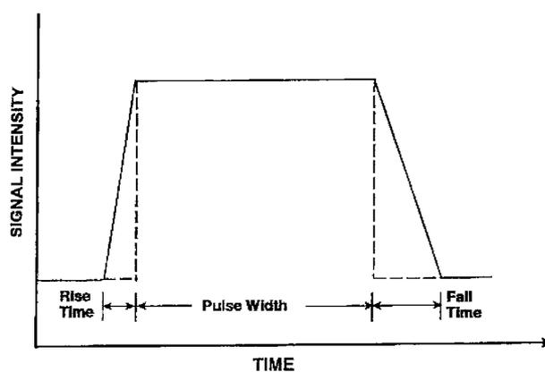
**Fig. 5** Trapezoid signal minimizes the problems with the rising time in case of rectangular signals
